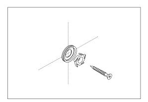
Fix SpinFix button and washer to substrate.
