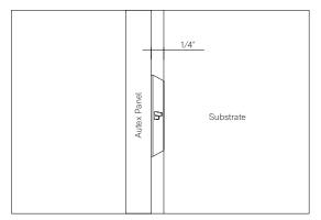
SpinFix clips create a 1/4" air gap for added acoustic performance
