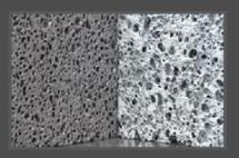
ALUSION™ Medium-Cell Cells Open on Two Sides (12.7 mm & 25.4 mm)
