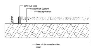
volume reverberation room: 214 m<sup>3</sup> surface area sample: 10,8 m<sup>2</sup> heigth of the construction: 0,060 m measured at: Peutz Laboratory for Acoustics signal: broad-band noise
